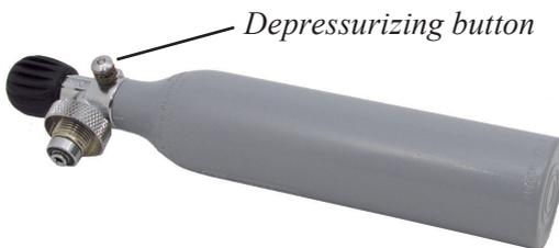
The Divator Rescue BC is equipped with a Rescue air inflation cylinder of 300 bar, 0,35 l volume. The cylinder is made of aluminium.
