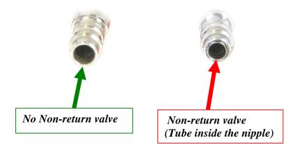
If the male coupling used together with the SCBA is without Non-return valve, no further actions is needed.
