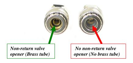
2. If the female coupling is without the brass tube it must be exchanged to the female extra air coupling with item number 95 244-01. Contact your local Interspiro representative for further information.
