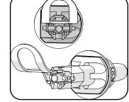
11. Assemble the valve insert with the new lever and lever support.
