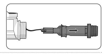
3. Remove the retaining ring and then pull out the valve insert from the connection nipple.
