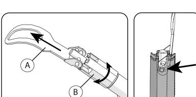
**IMPORTANT!** Never angle the lever more than 50 degrees as this may damage the contact surfaces on the lever support. When the valve insert is mounted in the breathing valve housing, the lever is prevented from angling more than 50 degrees. When the valve insert is removed from the breathing valve housing, the lever can be angled more than 50 degrees and thus damage the lever support.
