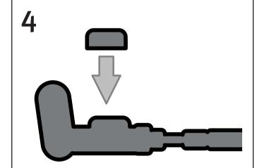
• Plug the breathing valve with the correct type of plug.
