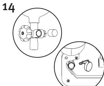
Remove any washing plug from the pressure gauge. 15
