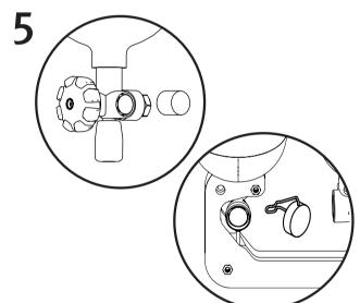
Plug the pressure gauge (if the cylinder / cylinder pack is equipped with a pressure gauge). 6 INDESSPERO
